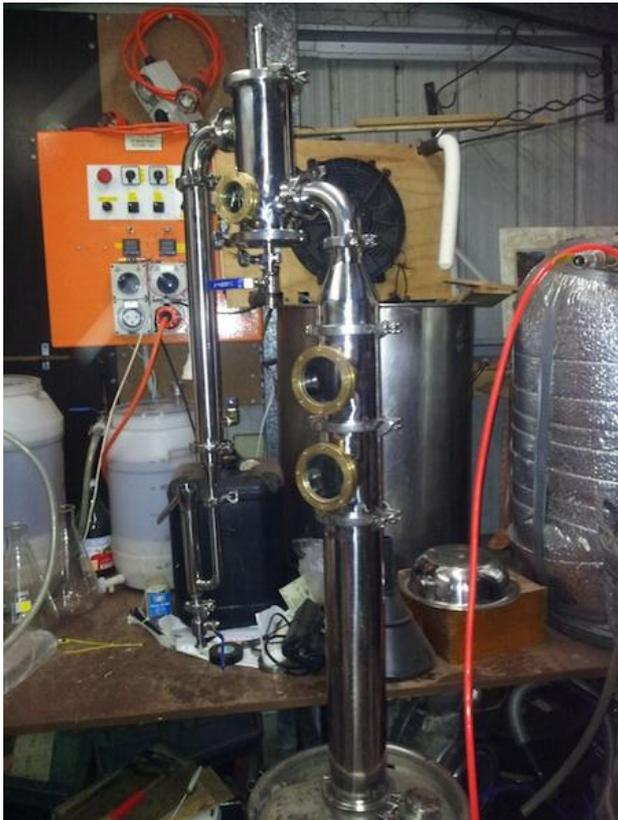
Figure 10: The Authors SD Gin Head adjusted to height using a 510mm section and 2 empty bubble Tees
