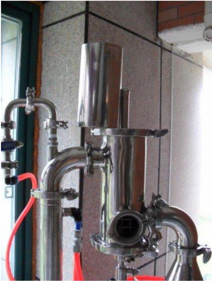
Figure 12: Standard Configuration with optional threaded 90° for clean in place
